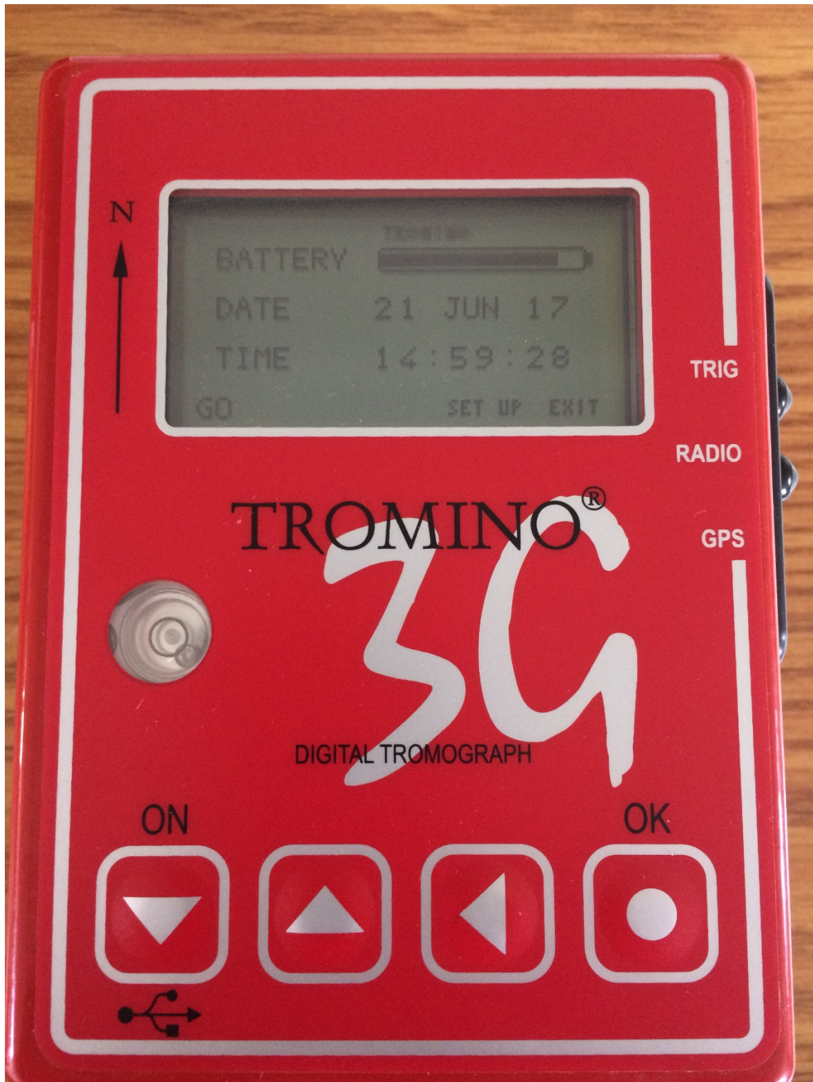
Tromino – first screen which appears, battery, date and time check.
