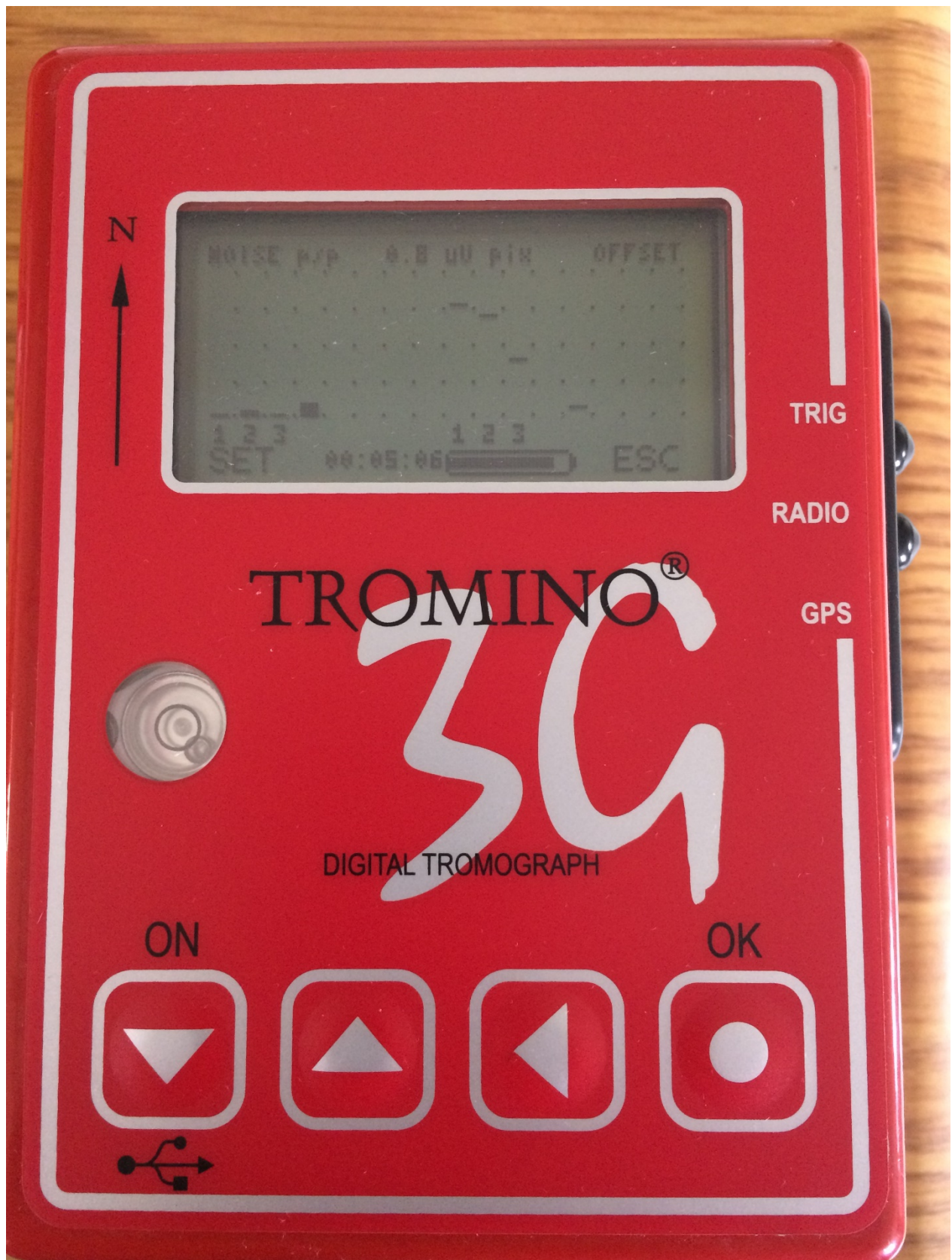
Amplifier Test, showing noise on each of the three channels (north-south, east-west and vertical)
